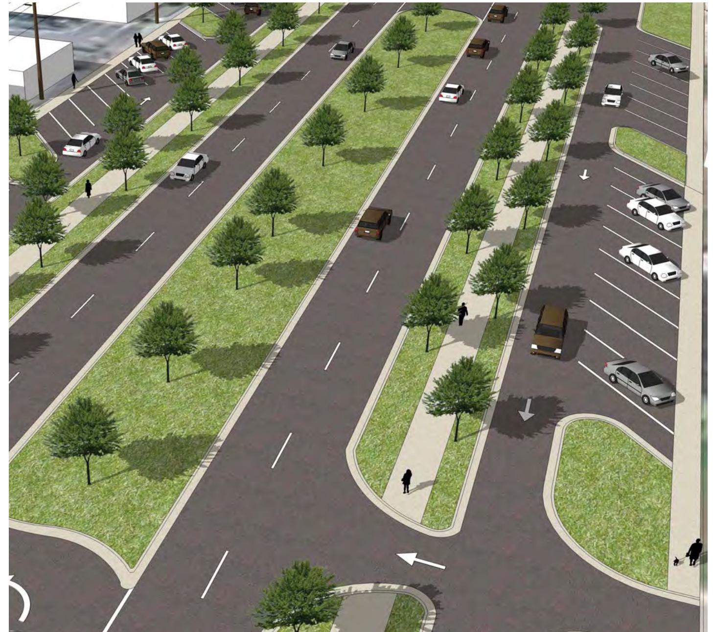
Figure 1.2.D: Roadway Perspective (showing reverse-flow parking)
